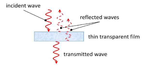
Figure 1. Interference in a thin film.
