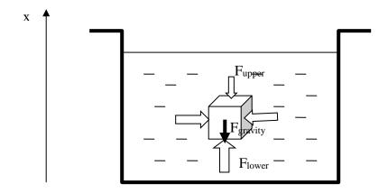
Let us consider a small cube of water inside the glass. The walls of this cube are imaginary, but the water inside is real. Since the cube does not move (the water does not flow inside the glass) the total net force applied to the cube is 0. We consider only the forces applied in vertical direction. There is a gravity force applied to the cube. It is:
