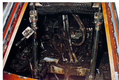
Figure 6: Apollo 1 cabin's interior after fire.
