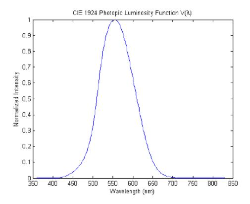
Luminous flux [lumens, lm] = 683 x  $V(\lambda)$  x Radiant flux [W]
